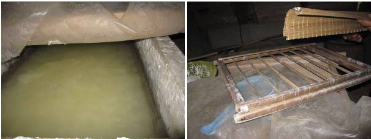
Pic 30. Pulp tank (left) and deckle and mould for making (right)
