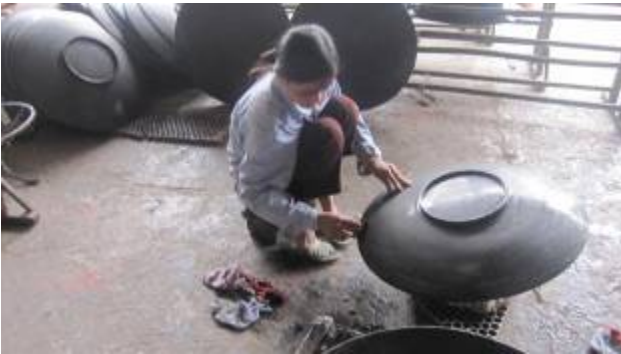
Pic 14. Coat cashew nut based paint to bamboo bowl
